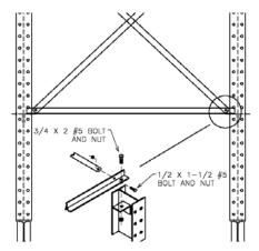
**D.** Now the balance of the uprights can be erected to complete the run. The uprights can be stood either one at a time or in groups of 2.
