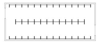
**B.** Snap a chalk line establishing the front edge of the upright bases. The chalk line should run the entire length of the row of rack.
